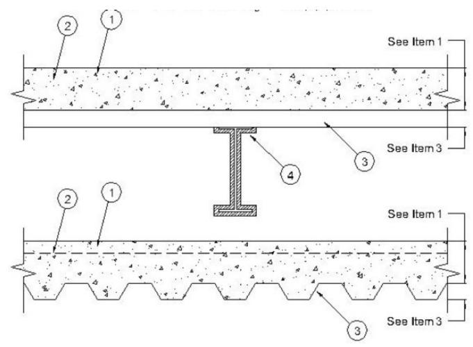
**Supports** — W8x28 min size steel beam or min.10K1 steel joists.
