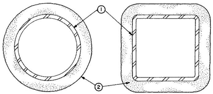
1. **Steel Pipe or Tube Column** — Steel circular pipe with diameter (OD) ranging from a minimum of 3 in. to a maximum of 32 in. with a minimum wall thickness of 3/16 in.
