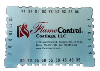
A wet film gauge like the one above can be utilized to determine the mil thickness of the paint film that has just been applied.
